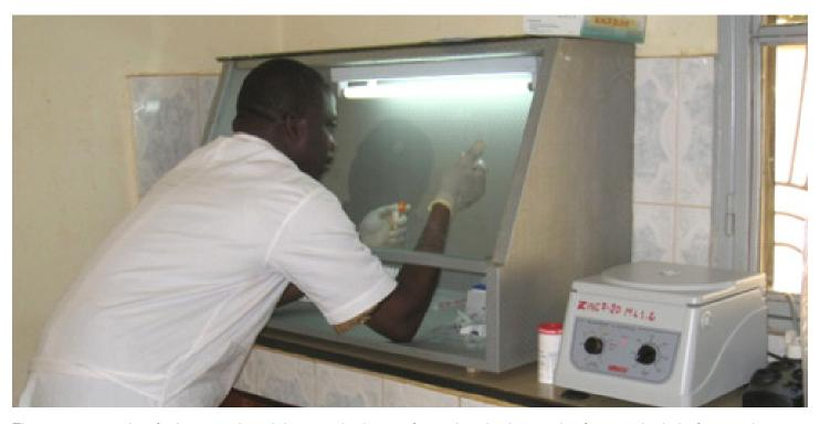
This is an example of a low-cost hood that was built out of wood, with glass in the front and a light for good visibility. The wood and all edges are carefully covered with a plastic wrap so that the hood can be easily cleaned with alcohol. When not in use, the hood can be closed with a removable glass.
