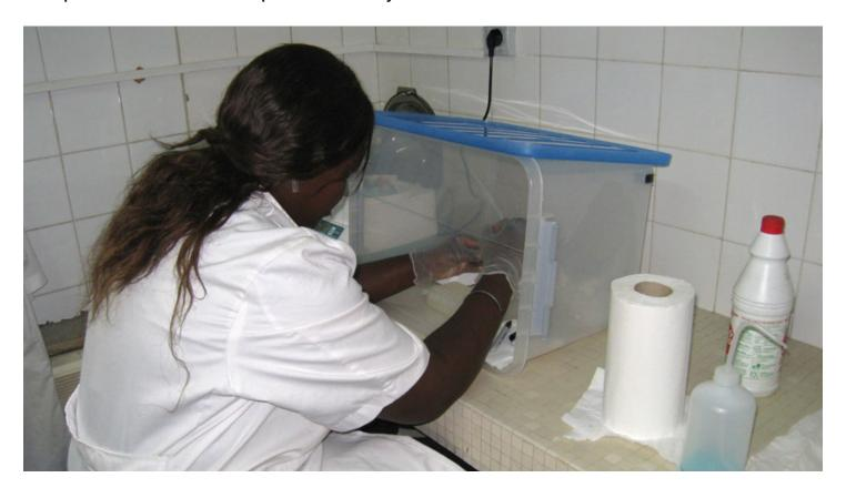
A simple storage box is positioned on its side. A plexi-glass cover was installed to cover the top half of the box to reduce the size of the opening. At the end of each day, the box can be easily cleaned with alcohol and stored with the lid closed to keep clean.
